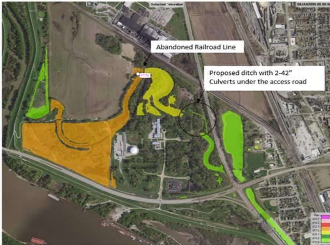
Figure -1 Inundation with 2-42" culverts placed at both the abandoned railroad line and the proposed ditch crossing, requiring a flowage easement of El 417.50 feet
