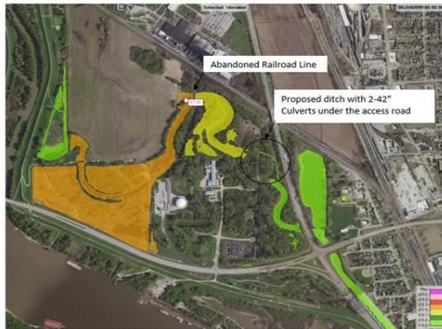
Figure - 2 Inundation with 2-42" culverts placed at both the abandoned railroad line and the proposed ditch crossing, requiring a flowage easement of 61 437.50 feet
